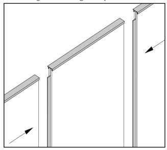
**NOTE:** The frame can be pre cut to each panel size and spliced at each board seam, or the frame can be shipped in bulk lengths and miter cut in the field for a full perimeter trim.
